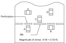
1-3. When breaking PC boards along their perforations, the amount of mechanical stress on the capacitors can vary according to the method used. The following methods are listed in order from least stressful to most stressful: push-back, slit, V-grooving, and perforation. Thus, any ideal SMD capacitor layout must also consider the PCB splitting procedure.
